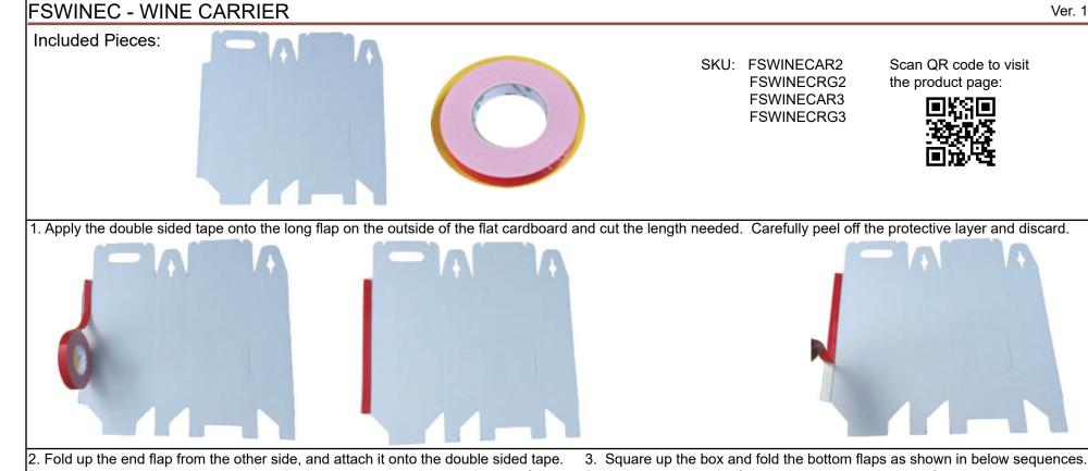
2. Fold up the end flap from the other side, and attach it onto the double sided tape Be sure the edge align with the cease. Apply pressure to make sure the tape fully contact with the cardboard and the edge is secure.
